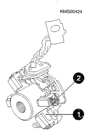
COMPONENT TESTING AND REPAIR Checking carbon brush wear Brush holder installation: Fit new brush holder in stator frame. If old brush holder is re-used, slip it back onto locating sleeve (1) from commutator and insert in stator frame. Ensure correct positioning of locking element (2). Brush holder
